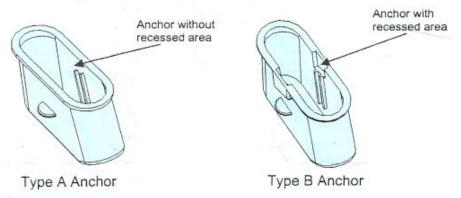
2. Place the wedge, wedge flat bar (wedge flat bar with boss is used on Type A Sockets only and the wedge flat bar without the boss is used on Type B Sockets only), washer, bolt, escutcheon plate and handrail in the anchor, respectively (refer to Figure below). If the flat bar with the boss is used, the boss shall face down in the anchor. Tighten the bolt down so that the handrail is secure in place.
