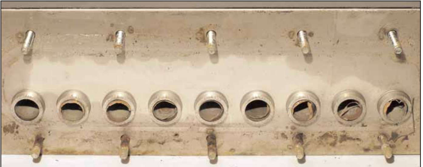
Ends of the tubes are worn thin.
