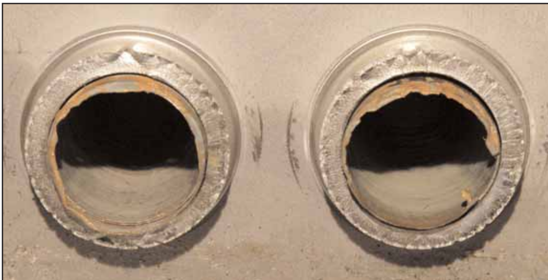
Ends of the tubes are worn thin.
