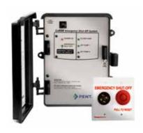
The Compool LX820 controller makes it easy and economical to enhance the safety of commercial spas. In the event of an emergency, pushing the mushroom-style button stops all spa equipment. This action shuts off the filter and up to two jet pumps, while sounding an alarm. Pulling the emergency button back out cancels the alarm, and returns the pumps to normal operation.
