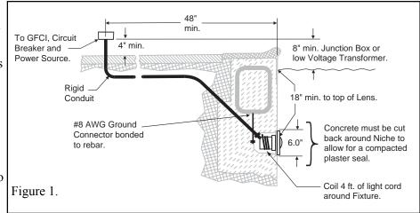
of the requirements of the National Electrical Code which the pool's or spa's electrical systems must meet are as follows
