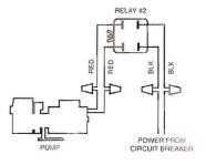
RELAY #2 (plugged into circuit board at JET1 socket).
