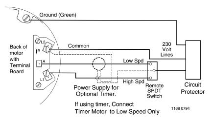
Minimum switch and timer amp rating must equal Branch Fuse Rating given in "Recommended Fusing and Wiring Data" table.
