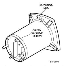
Figure 3 - Typical ground screw and bonding lug locations.
