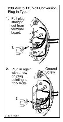
Figure 4B – Wiring connections for plug-in type terminal board (single speed, single phase motors).
