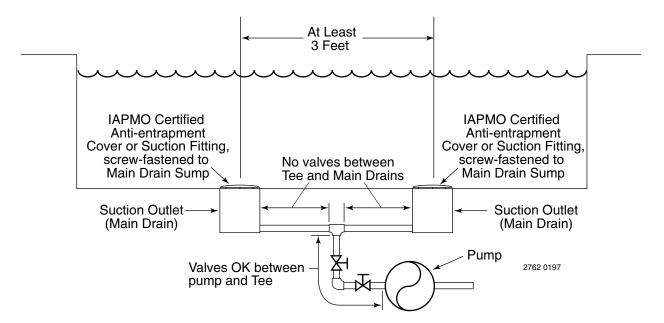
Figure 2 – Recommended pump suction layout.
