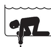
**Pool and spa pumps move large volumes of water, which can pose extreme danger if a person's hair comes in close proximity to a drain that is not the proper size for the pump or pumps.**
