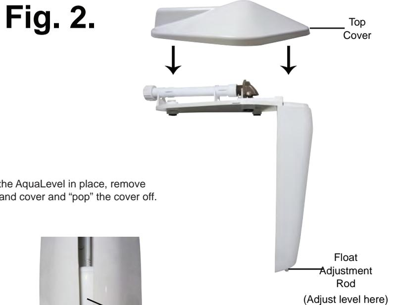
NOTE: If top cover has been installed and weight needs to be added to keep the AquaLevel in place, remove lid with a flat screwdriver. Put the end of the screwdriver in between the base and cover and "pop" the cover off.
