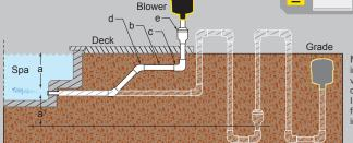
NOTE: Include a¹ for stallations with a check valve below the air outlet only. See "Below Grade Installation" on facing page for details. For above grade installations enter 0 for a<sup>1</sup>.
