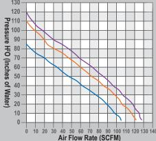
Locate the total back pressure, calculated above and draw a horizontal line. Locate the total airflow from previous step and draw a vertical line. These lines will intersect on the performance curve of the minimum HP blower required for your application.
