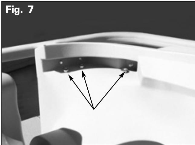
These 3 locations receive a flange nut and a rubber cap. A flat washer is not needed. Hand tighten.
