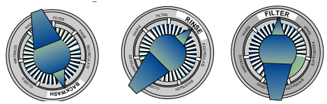
Fig. 9: Valve settings for startup. Stop pump before changing valve position.
