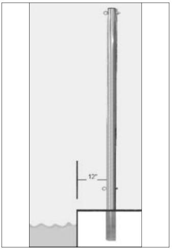
**Figure 4** Deck Anchors should be set back 12" from pool edge
