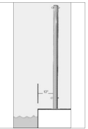
Figure 6 Poles should be set back 12" from pool edge
