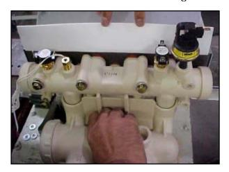
9. Install the temperature sensing probe by passing the wires through the hole provided on the left side of the brace panel. Route wires through the support bracket.
