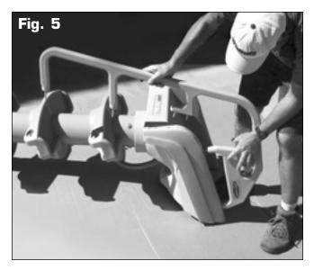
Insert handrail into the top section first as illustrated. Push or pull the handrail apart until the all-threads pass through the 6 holes.
