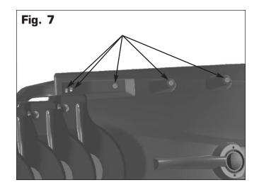
These 5 locations on the entry section receive a flange nut only. A flat washer is not needed. Hand tighten.
