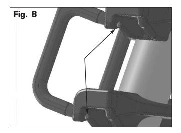
These two locations require a flat washer, flange nut and rubber cap. Hand tighten.
