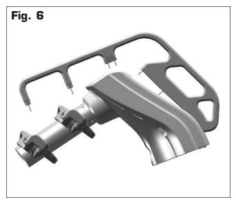
Insert handrail into the top section first as illustrated. Push or pull the handrail apart until the all-threads pass through the 5 holes in the entry section and through the holes drilled in the upper 2 steps.
